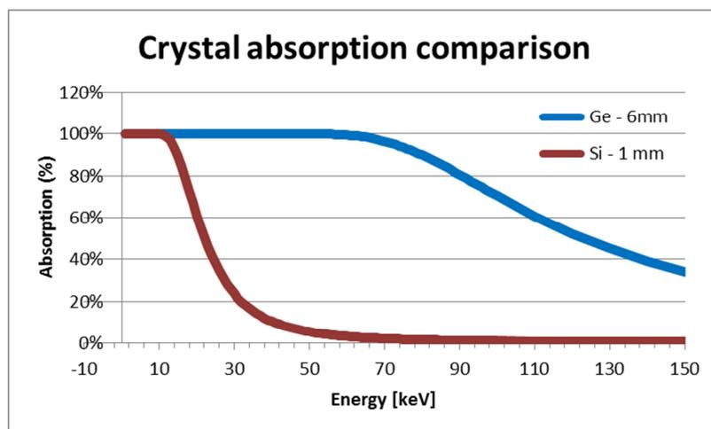
Fig. 3 - Comparison of crystal photoelectric absorptions for 6mm thick Germanium as well as 1mm thick Silicon (Silicon diodes are usually between 0,5mm and 1mm thick). HPGe is the most appropriate technology after 15keV
