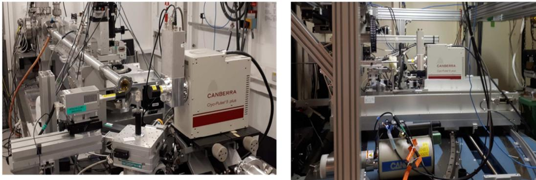
Fig. 1 - CANBERRA single element detector for performance testing at ESRF (BM23) for an EXAFS experiment and at Spring8 (BL04) on an energy-dispersive diffraction experiment
