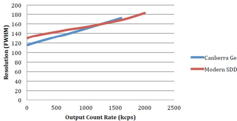
Fig. 5 - Energy resolutions of the HPGe demonstrator compared to a SDD of similar sensitive area (by courtesy of Quantum detector)
