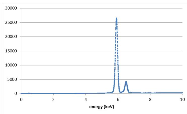
Fig.4 - Example of spectrum recorded with a Fe55 source at 550kcps at the detector, with a Canberra Lynx® digital MCA. The Gaussian shaping time is set at 0.1µs and the FWHM at 5.9 keV is 150eV
