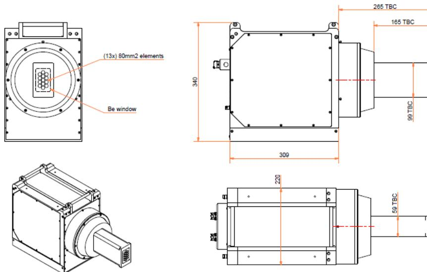
Fig. 8 – Example of 17 element detector array design, electrically cooled
